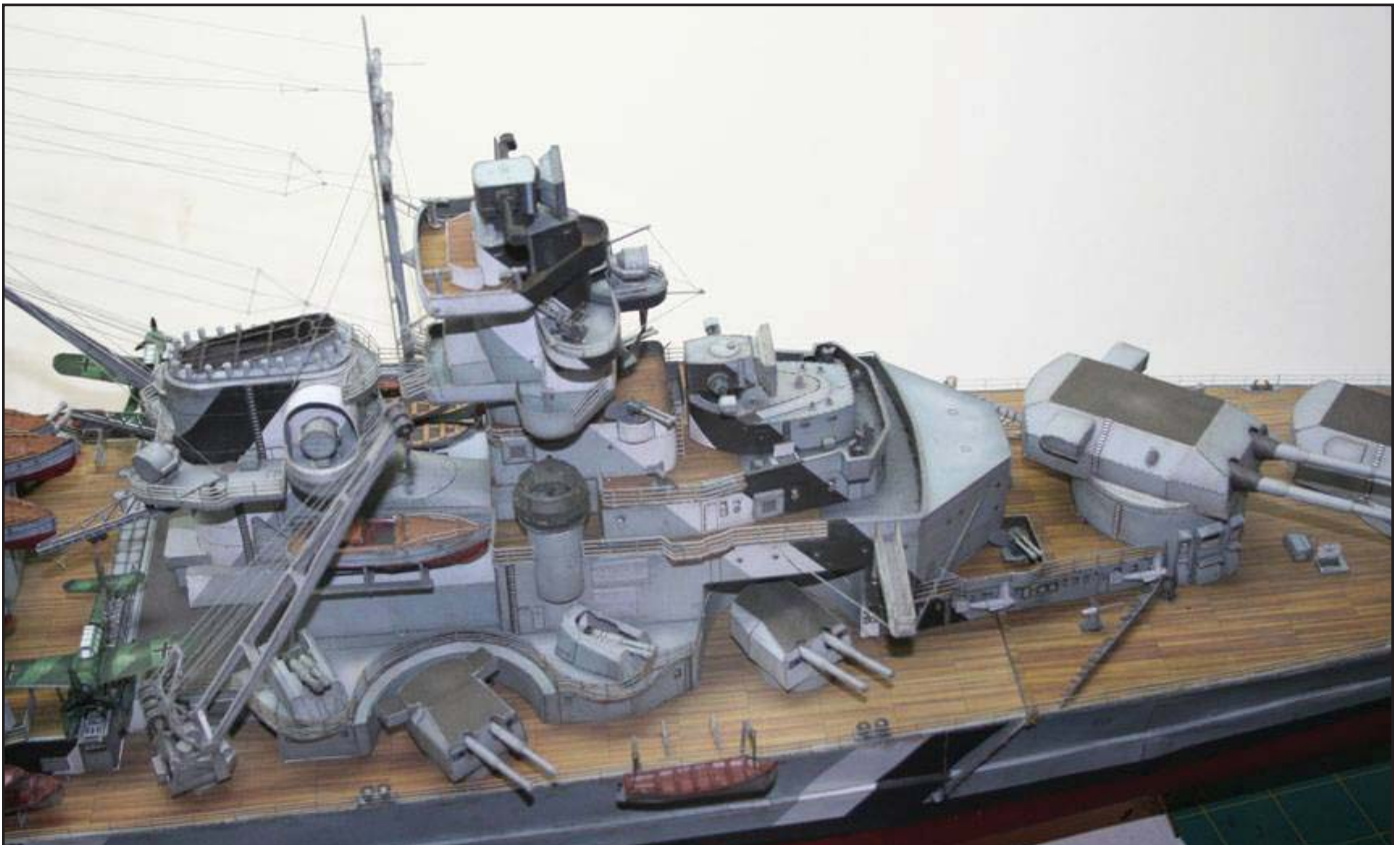
16 & 17. DKM Bismarck , 1:200 scale, published by GPM (Poland) Built by David Sakrison, the Bismarck model includes etched brass railings on the main deck, masts of steel wire wrapped in paper, and main gun barrels redrawn in Photoshop. Everything else is paper. David has posted brief tutorials on the hull, gun barrels, and rigging at www.papermodelers.com . GPM also has a kit for Bismarck 's sister ship, Tirpitz . Photographs by the author.
